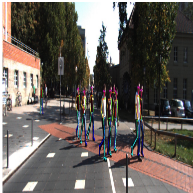
Figure 2.5: Result of OpenPose joints detection. The training sequences number 16 of the KITTI tracking benchmark.
