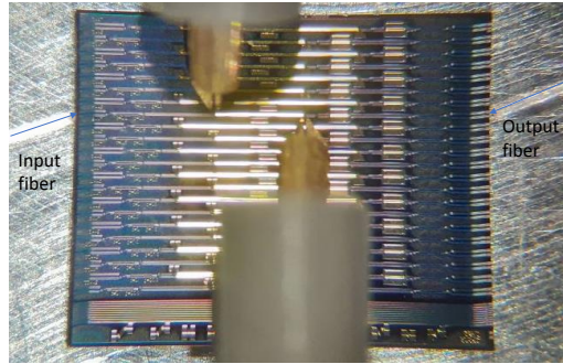
Figure 4.6: Photonic integrated circuit cell including 22 modulators under electro-optical measurement
