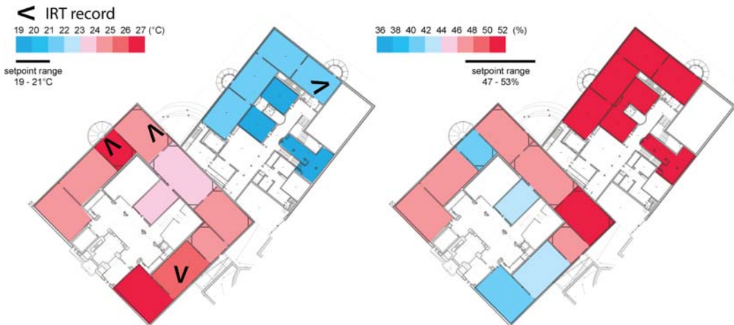
Figure C.11: Averaged short-term measurements for T (left) and RH (right) for the ground floor of M3. Measurements were performed on July 20, 2016. External climate data: T_{average} was 26.4°C ( T_{max} = 33.9^\circ C , T_{min} = 20.2^\circ C ), RH_{average} was 41.7%.
