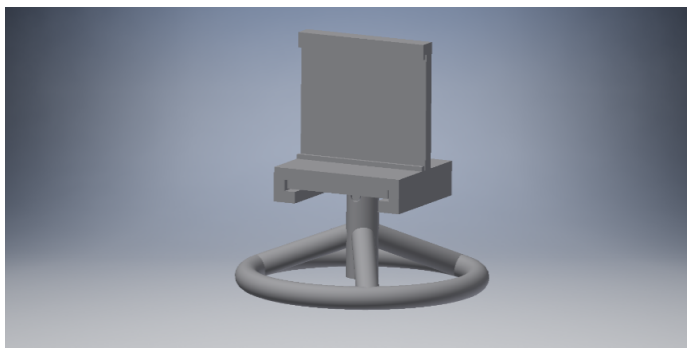
Figure 5.3: Depiction of the 3D-printed sample holder in the vertical position.
