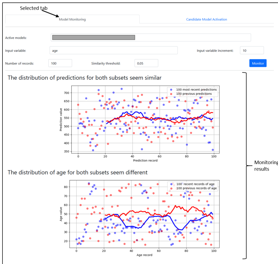
Figure 13: Webapp tab that shows the model monitoring engine functionality of the prototype. The name of the active model being monitored is hidden behind a gray rectangle due to privacy policies.
