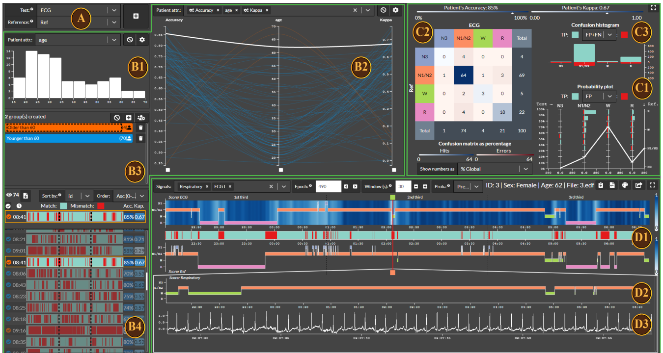
Figure 3: The views B1-B4 are patient-related, where B1 and B2 depict views where patients can be filtered based on the selections performed. B4 displays the patients that match the current selection. Groups of patients can be created, modified and selected in B3. C1-C3 shows performance information, where C1 depicts our probability plot, C2 a confusion matrix and C3 complements information displayed in the confusion matrix. In D1 the physiological data view shows the hypnograms for a selected patient. Alternatively, extra models can be visualized together with those selected in A as shown in D2. Finally, D3 shows the signals that represent the input data.
