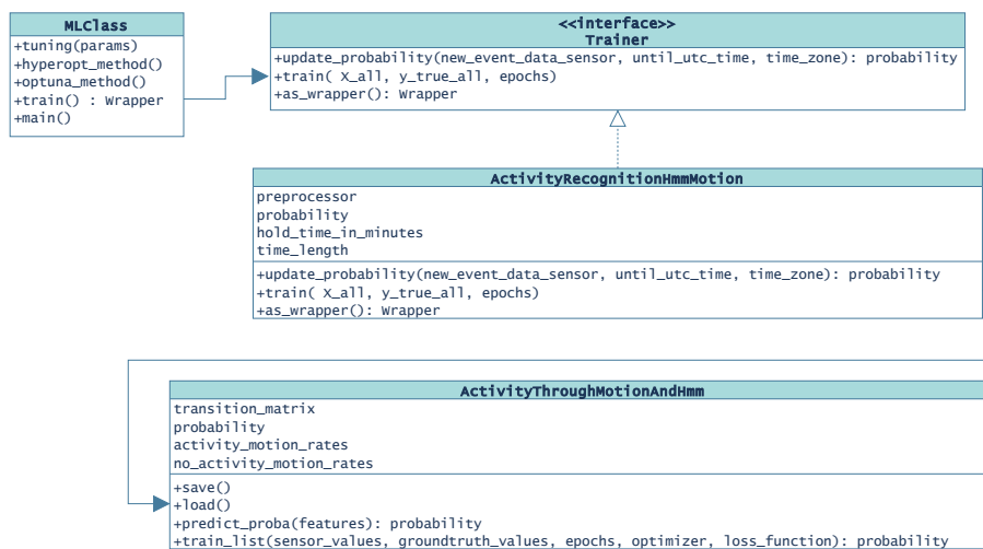
Figure 5-8: Adapter design pattern enables using third party training libraries for pipeline
