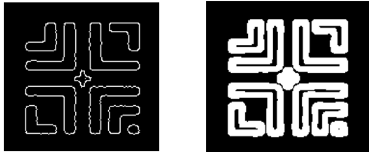
Figure 59. Initial image (left side) and dilated image (right side)
