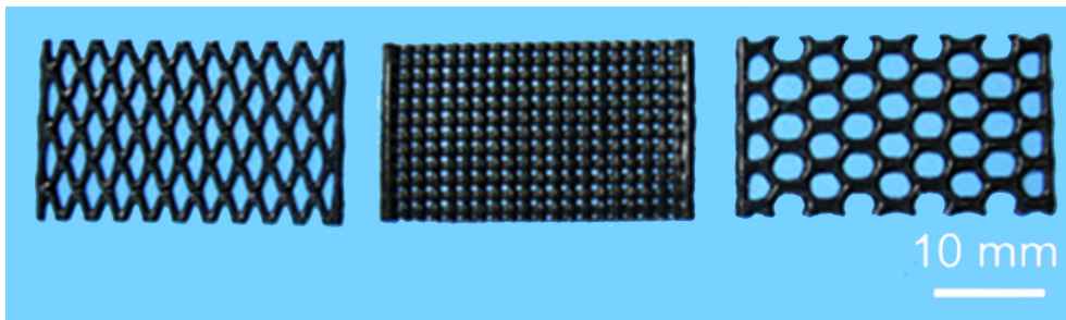
Fig. 4-16. Different structures of printed M-PDMS-G composites.
