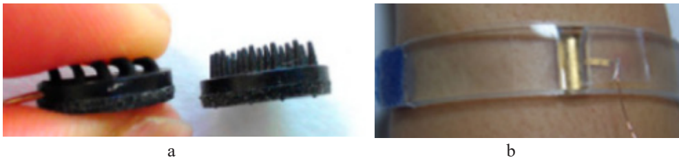
Fig. 2-3. (a) Conductive polymer dry electrodes based on EPDM[68]; (b) conductive polymer dry electrodes based on PDMS[69]
