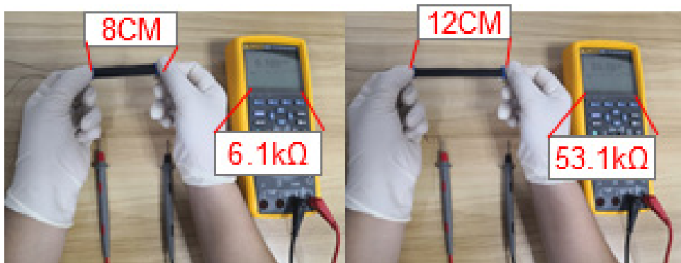
Fig. 3-9. Resistance change while PDMS-Graphene compound is stretching. The original state of material (right); The stretched state of material (left).
