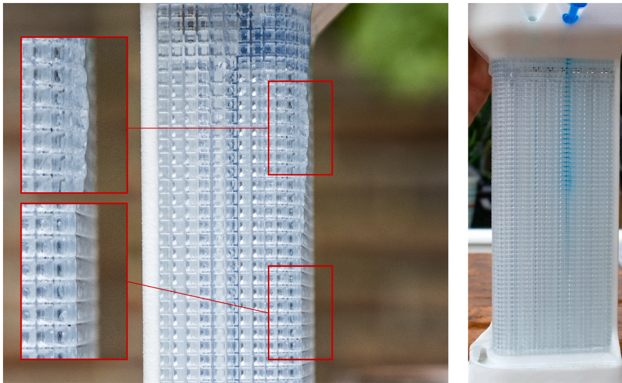
Fig. 10. Photograph of the water flow experiment in progress. The water flow is homogeneous and stable across most of the surface. Overflowing is only observed where the CPS curves around the corner, and near the water inlet.
