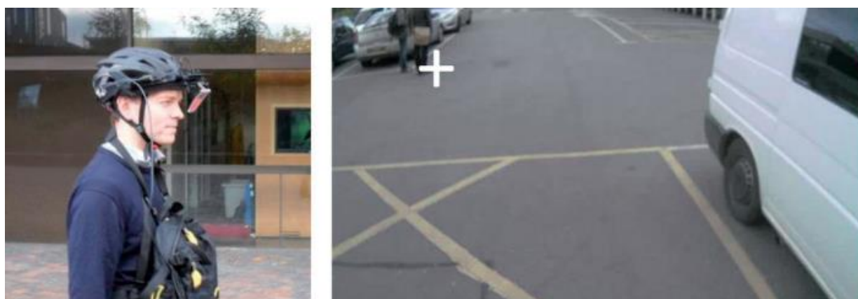
Figure 2-16: iView X HED mobile eye-tracking system (left) and screenshot from a recorded video (right). The white cursor indicates the gaze location (Fotios et al., 2015)
