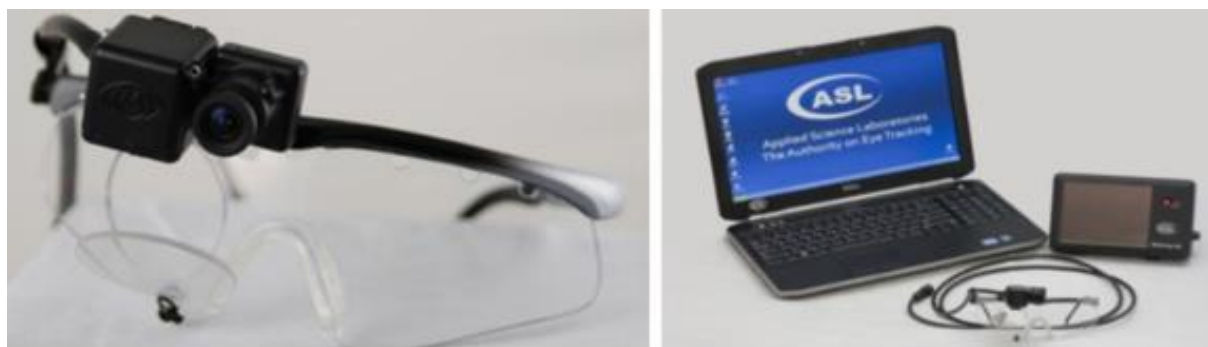
Figure 2-17: ASL Mobile Eye XG Glasses on the left, complete equipment on the right (Mantuano et al., 2017)
