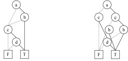
(a) Variable order a < b < c < d (b) Variable order a < c < b < d
