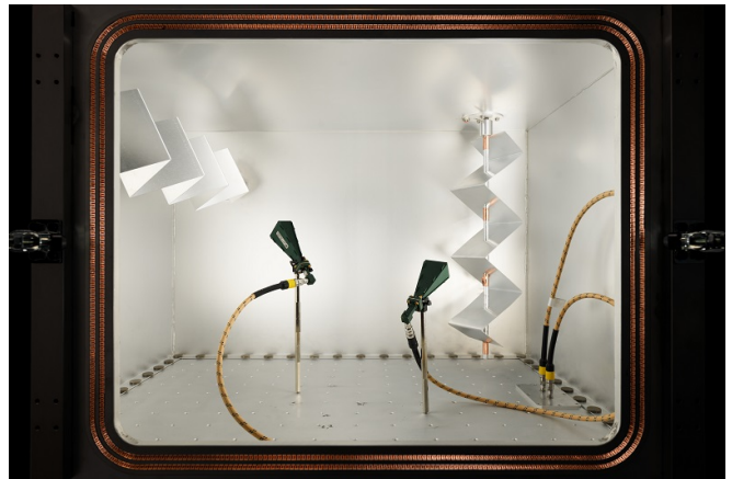
Fig. 1. Novel mm-wave reverberation-chamber with a setup for 20-40 GHz.
