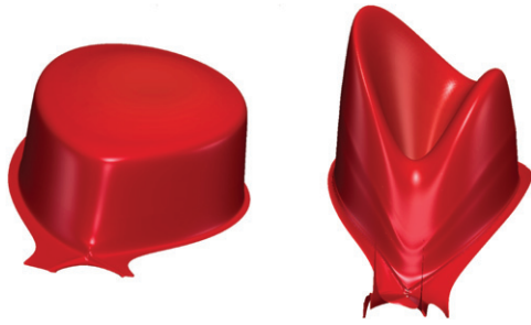
Figure 12. Example of the G^1 continuous, i.e., continuous values and first derivatives in real space, profiles in the poloidal plane for (left) a density distribution and (right) the perpendicular conductive heat flux.
