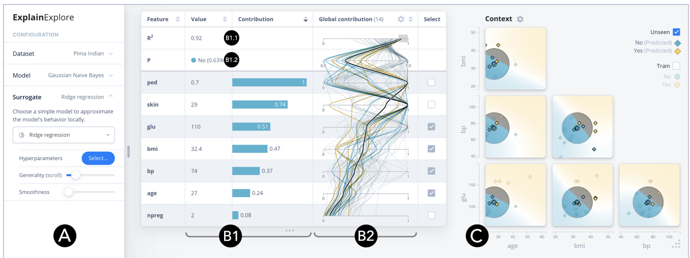
Figure 4: Graphical user interface of EXPLAINEXPLORE showing the main components: (A) the configuration view to select and refine model and surrogate parameters; (B) the feature view explaining the prediction by (B1) showing feature-wise contribution values for one case using the chosen configuration, and (B2) providing a global overview to identify whether the selected instance was classified similar to other instances, or whether the model has ‘strategies’ specific to a subset of instances, and (C) the context view showing neighboring instances, the class probability gradient to assert whether the surrogate model is accurate, and allowing to explore the effect of instance perturbations.
