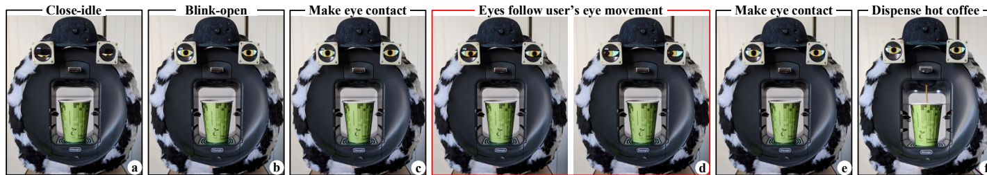
Figure 28 Eye-follow condition: (a) From close-idle, the coffee machine (b) eyes blink-open, (c) make eye contact with the user, (d) interact by following the user's eye gaze, (e) make eye contact again, and (f) dispense coffee if the user stays engage for 3.5 s.
