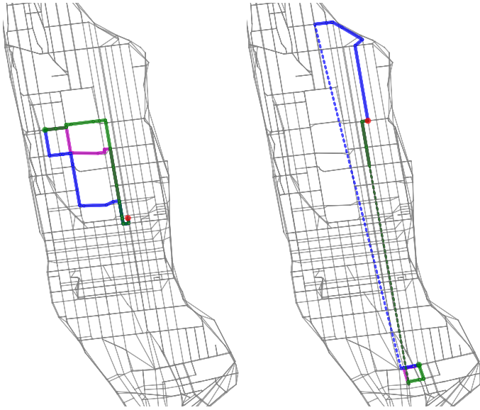
Fig. 8. Example of the SO routes connecting an OD pair. Green and red dots represent origin and destinations, respectively. Solid lines portray traveling flow in the road network while dotted lines describe flow traveling via subway.
