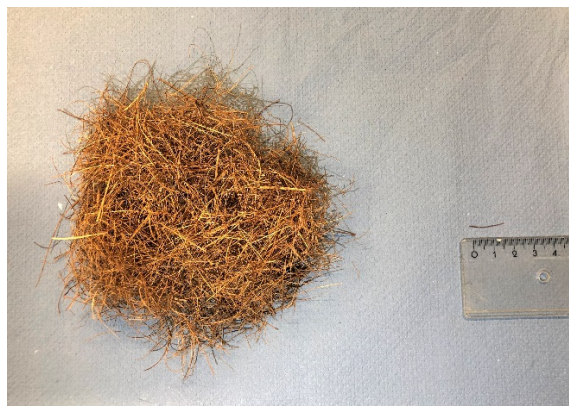
Figure 4. Appearance of coir fibers. The average length of coir fibers is about 15 mm.
