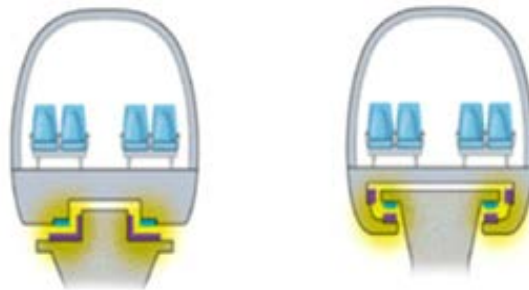
Figure 1. (Left) Electromagnets on the guideway levitate the car; (Right) Electromagnets on the cars lift the cars.
