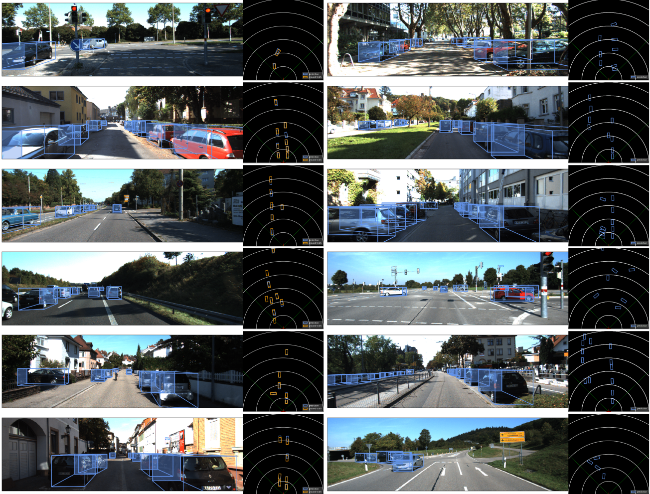
Figure 6. Qualitative examples from the validation (left) and test (right) sets in KITTI. The non-transparent side of the bounding box represents the front part of each car. Bird’s eye view is also provided to show that SMOKE can recover object distances accurately. Note that all these images are not included in the training phase.
