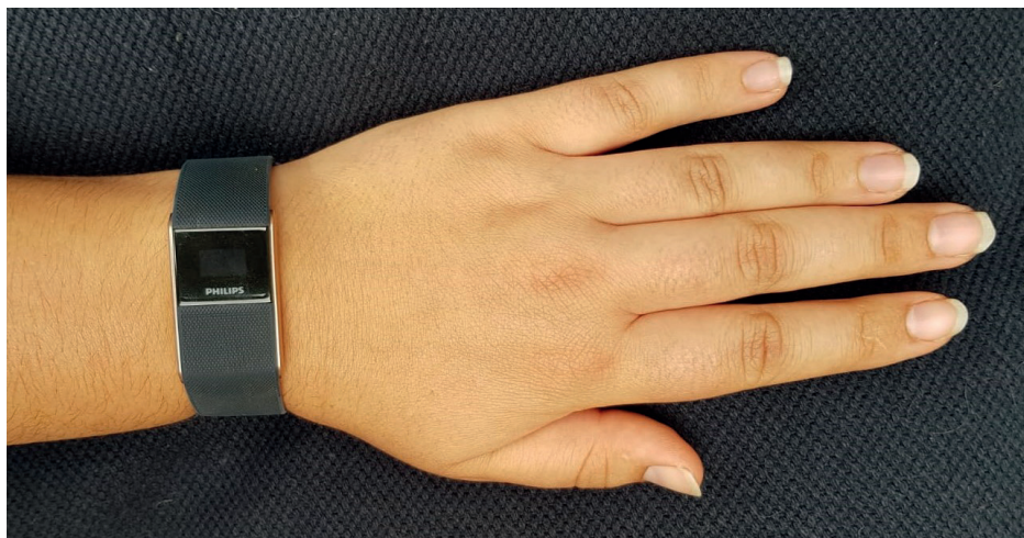
Figure 1: The Philips Data Logger. This device will be employed in this study to acquire PPG and accelerometer data. The device does not display this PPG and accelerometer data, it only displays the time.
