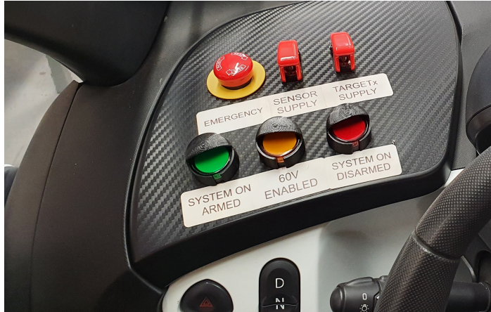
Figure 2.6.: Operator panel for the fallback-ready user with LEDs to indicate the automated control system status
