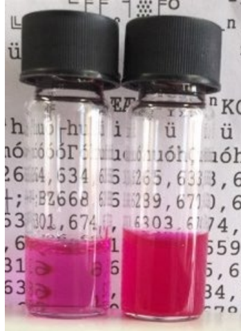
Figure S1: The concentrated 30 nm RITC-SNPs dispersion in water (right) and in 80 vol% (83 wt%) glycerol and 20 vol% (17 wt%) water mixture (left). The SNP dispersion became nearly transparent by the refractive index matching.
