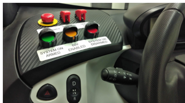
Figure 2.2: Twizy 2 operator panel [107]
