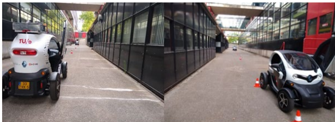
Figure 47: Static Test Setup with cones placed at steps of 10m.
