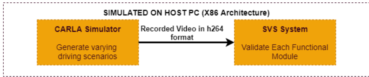
Figure 43: CARLA Simulator setup for unit testing of SVS functions
