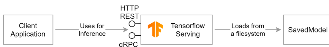
Figure 31: TensorFlow Serving serves an ML model to a client application
