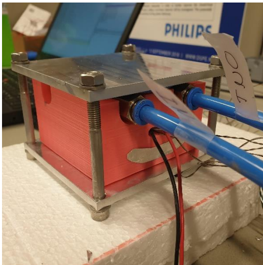
Figure 1 Experimental setup used for the calibration of temperature dependent parameters.
