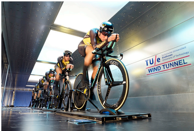
Fig. 11. Wind tunnel tests of a team time trial in the closed-circuit wind tunnel with closed test section at Eindhoven University of Technology in the Netherlands (photo by Bart van Overbeeke; reproduced with permission).
