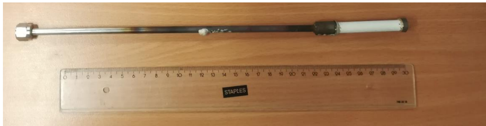
Figure 5.1. Picture of the sealed (by means of the RAB sealing technique) MgO porous membrane used to carry out the membrane reactor experiments.
