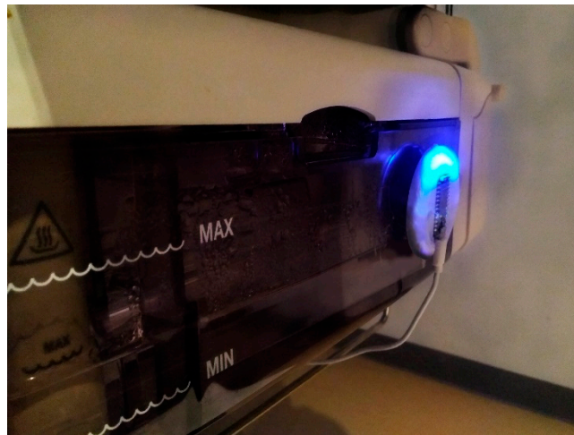
Figure 1. CheckMate attached to one of the medical devices; the water container of an incubator.
