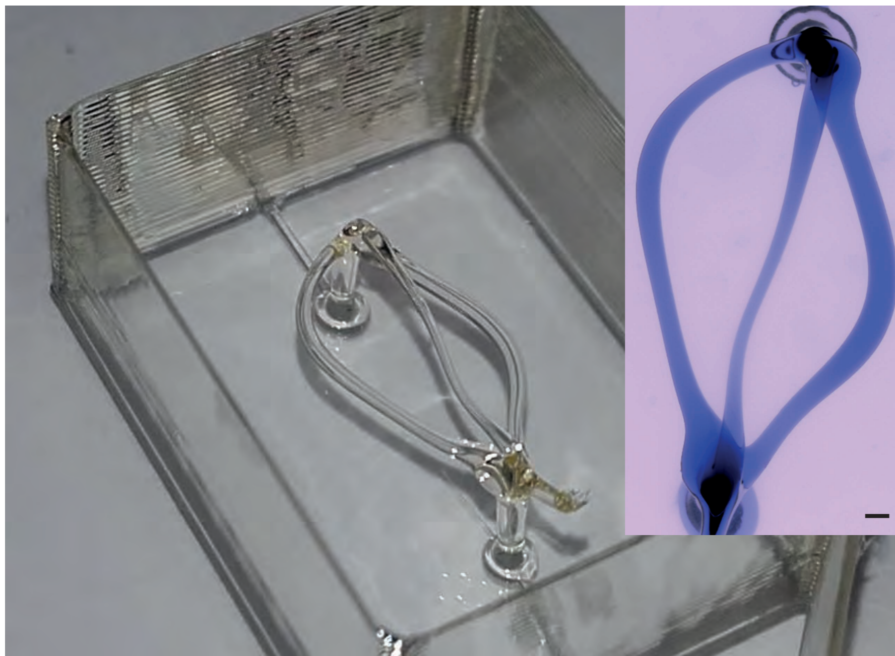
Fig. 1: Free-standing structure of sugar glass inside a printed casting frame mimicking the vascular architecture. Inset: Perfused network with dye solution after dissolving sugar glass cast in PDMS. Scale bar 500 \mu\text{m} .
