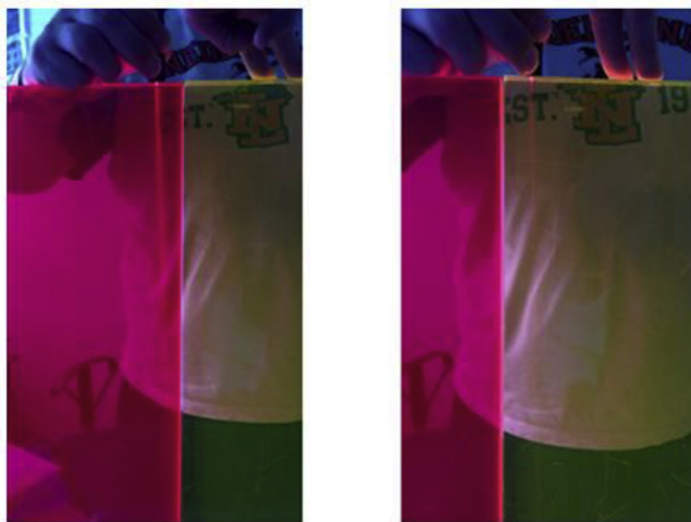
Fig. 6. Photograph demonstrating scattering of red laser pointed beam by (left) Red305 plate and (right) Orange240 plate from the same noise barrier. (For interpretation of the references to color in this figure legend, the reader is referred to the Web version of this article.)
