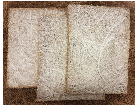
Fig. 13. The cement-coir composites made for the different conditions.
