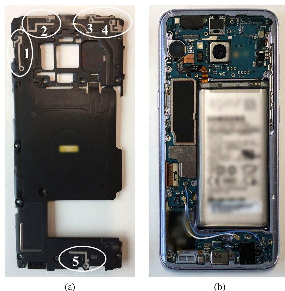
FIGURE 2. The smartphone partly disassembled. The antennas (a) consist of metallization on two pieces of plastic, that are normally mounted in the same orientation to the rest of the phone (b). The phone's boards connect to the antennas using spring fingers.
