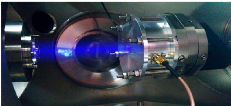
**Figure 1.** Photograph of the inner side of an experiment chamber in which a low pressure (argon) gas is irradiated with a pulsed beam of Extreme Ultraviolet (EUV) photons. The blueish glow at the position where the EUV beam travels indicates the interaction between the EUV photons and the gas.
