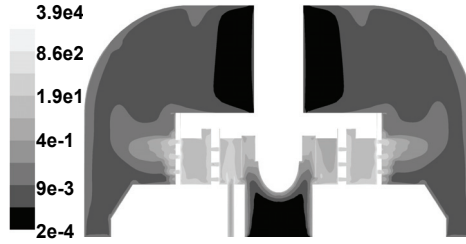
Fig. 5. Results of simulations of the flow in the rotor-stator mixer. Rate of energy dissipation [ \text{m}^2/\text{s}^3 ] distribution for Q=1.0 \cdot 10^{-4} \text{ m}^3/\text{s} , N=16.7 \text{ s}^{-1}
