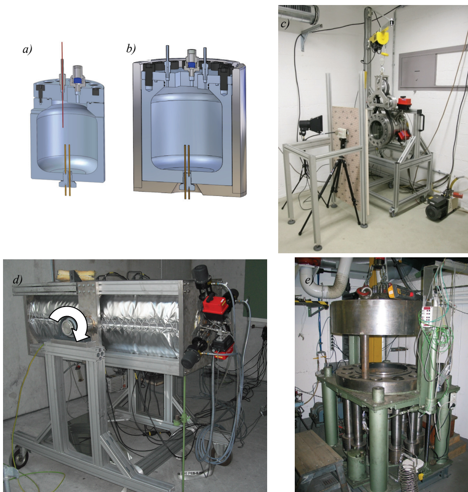
Fig. 1. a) Cross-section of the 3.0 L vessel, b) cross-section of the 6.5 L vessel, c) 10 L vessel with a window, d) 100 L vessel placed in a rack in order to change orientation (horizontal or vertical), and e) 50 L spherical vessel.
