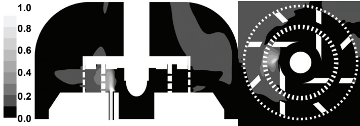
Fig. 7. Results of simulations of mixing in the rotor-stator mixer. Mixture fraction distribution for Q=1.0 \cdot 10^{-4} \text{ m}^3/\text{s} , N=16.7 \text{ s}^{-1}
