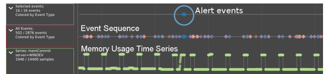
(a) Moving average of memory usage was above threshold (30GB), triggering alerts. The alert events are shown in the top sequence.
