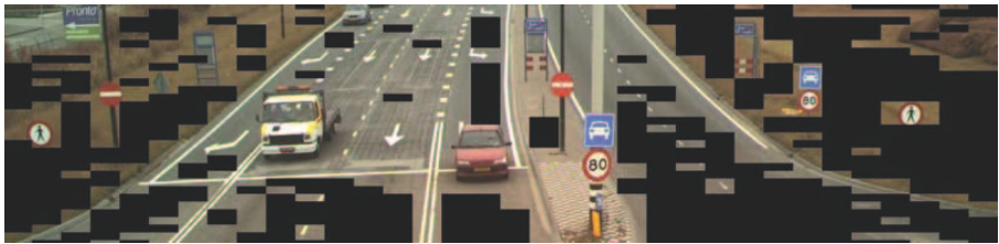
(c) Our DCT-based salient region detection approach
