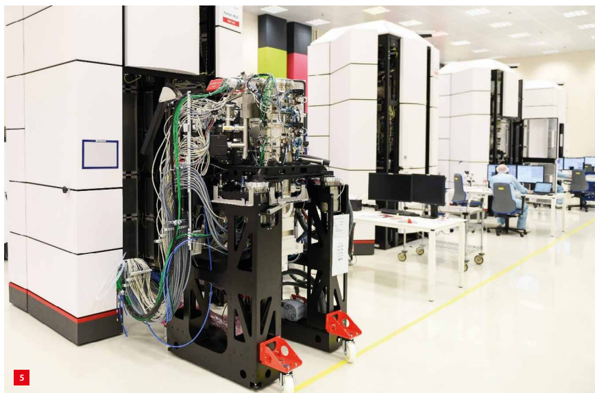
Thermo Fisher Titan microscope outside an opened acoustic enclosure. (Photo: Leo Koomen)
