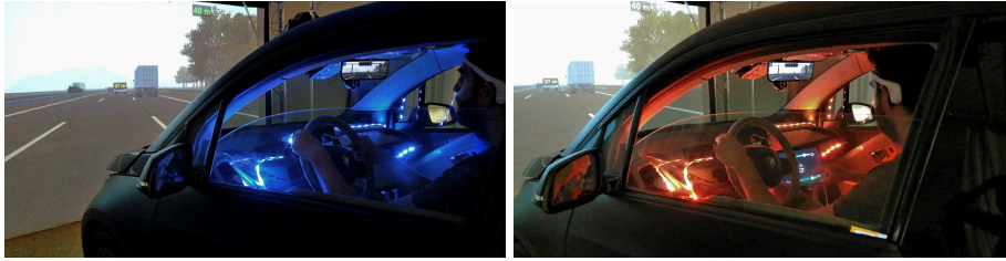
Fig. 1. A driver in our simulator study to evaluate our concept, wearing the EEG and heart rate sensors during the blue (left) and orange (right) ambient lighting conditions. The sensors were used to detect the driver’s emotions while the ambient light was used to influence driving behavior. Both light colors improved driving performance compared to a baseline ride due to their warning (orange) and calming (blue) effects.
