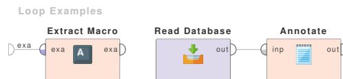
Figure 4.12: RapidMiner subprocess to extract each table when connecting to a SAP database
