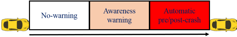
Figure 3.2 – Notification levels for safety application
