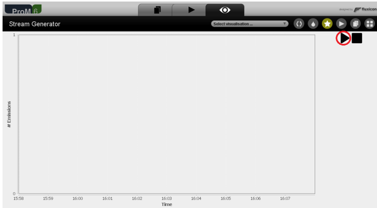
(a) Visualization of the Stream Generator object in which the stream is inactive. We are able to start the stream by clicking the play button in the top-right of the visualizer, highlighted by means of a red circle.
