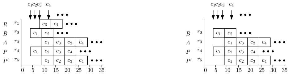
Fig. 5: Example execution schedule for the Petri nets in Fig. 3. On the y-axis, we have the tasks with the resources ( r_i ). On the x-axis, we have the time. The c_i s are the cases and the small downward arrows are the arrival of cases.
