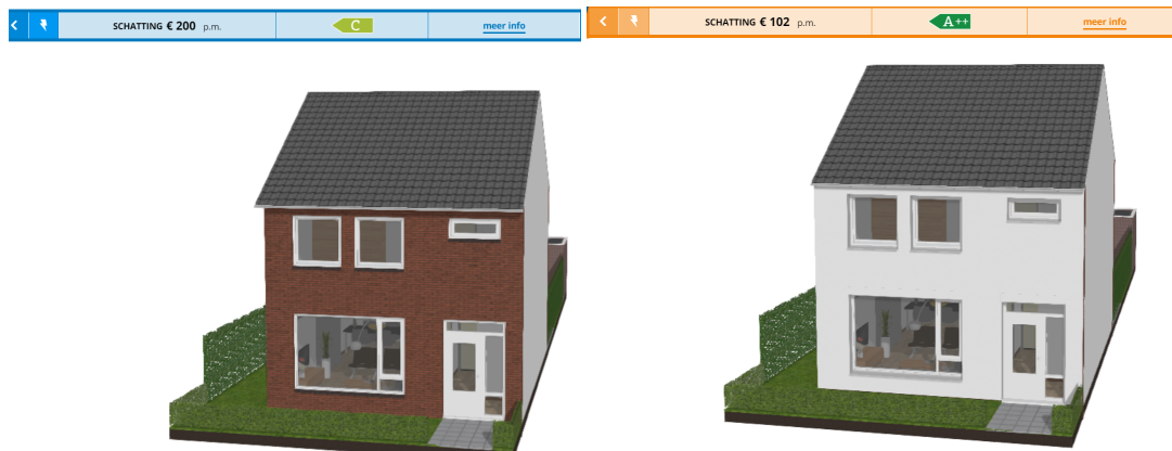
Figure 33: Example of how the visual BIM-model is adjusted after the renovation options have been selected (new insulation for the outer wall was added). The model also provides direct feedback on the costs per month and the energy label.
