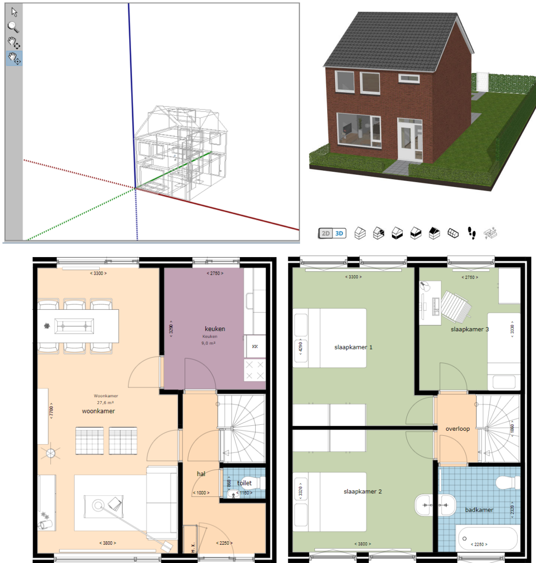
Figure 20: Overview of the BIM-model made in WoonConnect. The upper figure shows the 3d model created in WoonConnect BIM-environment. The lower figures shows the resulting floor plans for the first and second floor.
