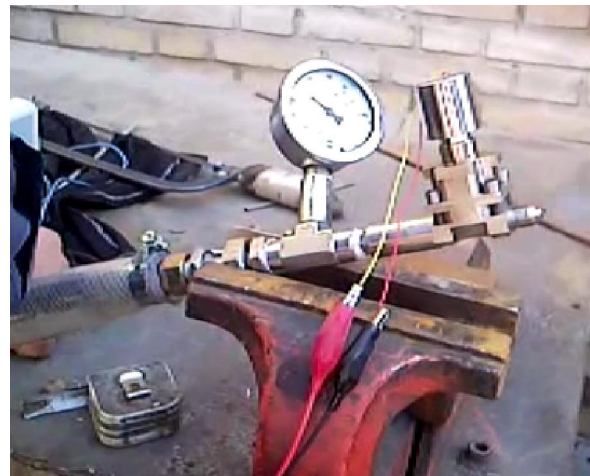
Fig. 6 Solenoid valve under operational tests.
