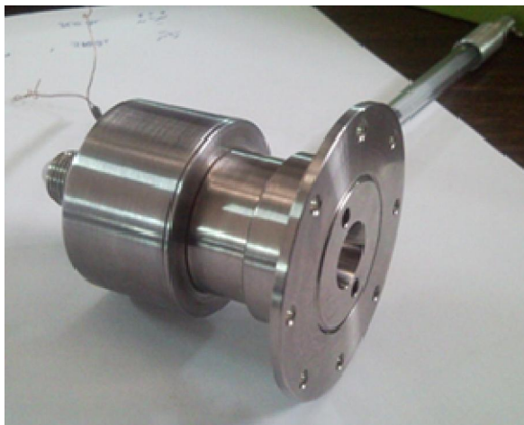
Fig. 1 Photograph of cold gas thruster and solenoid valve as one unit.
