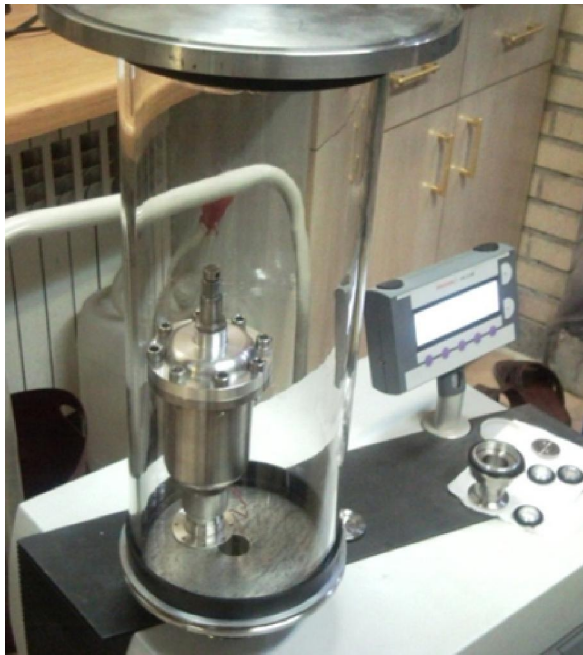
Fig. 6 Thruster leak test with helium in mass spectrometer.
