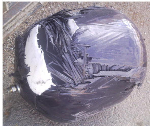
Fig. 5 Photograph of Tank burst at 730 bars.
