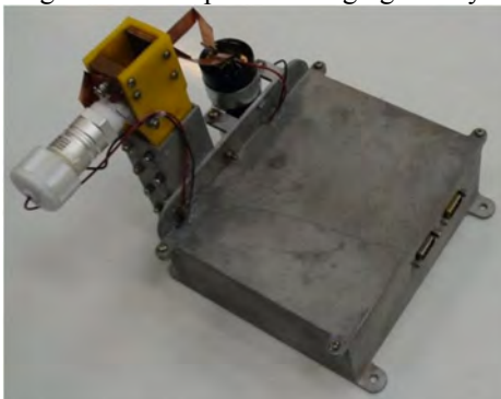
Fig. 9 The compact Eng-model PPT, its PPU inside and capacitor mounted on the case.
