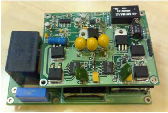
Fig. 7 PPU designed on a two-floor board.
