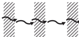
Figure 4.15. Schematic presentation of the considered diffusion concepts for wood. The striped regions represent the cell wall fibers, while the blank regions represent the lumen or other void spaces.
