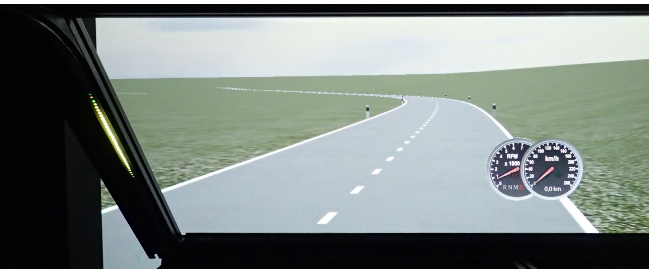
Figure 6. Ambient Light concept implemented on the A-pillar of the driving simulator. The greenish LED segment on the left is moving from the bottom to the top of the A-pillar and then past the driver, in the peripheral view of the driver.
