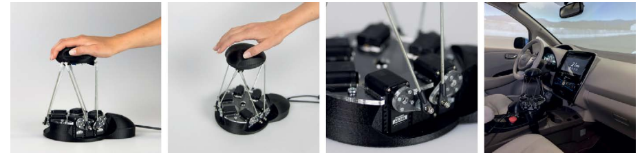
Figure 7. Stewart II, a future concept that allows for a haptic dialogue between an intelligent self-driving car and driver [Ros, 2017]
